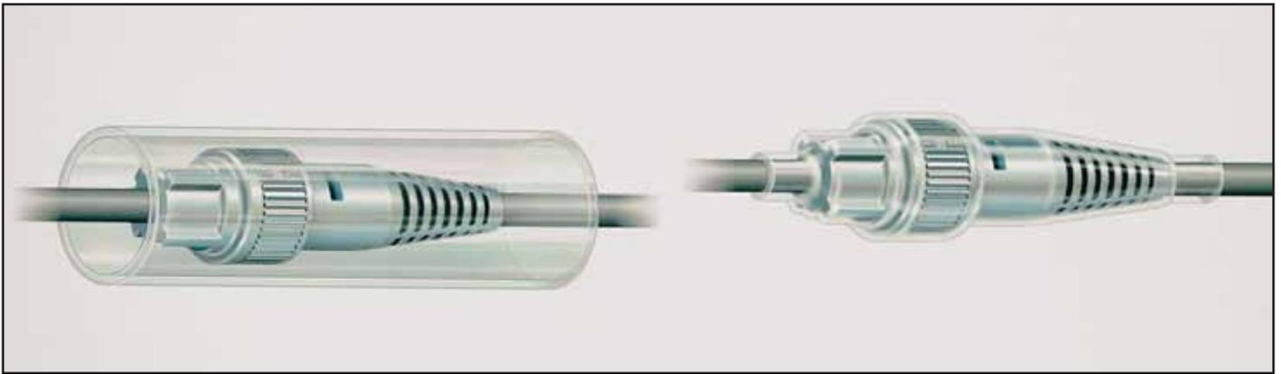
ZEUS Dual-Shrink® tubing of fluoropolymer PTFE/FEP is constructed with an exterior of heat shrink PTFE and an inner layer of FEP. It is easy to apply, and is designed to provide a tight, moisture-proof bond over wires, cables, connectors, splices, terminals, etc. The PTFE shrinks tightly over inserted parts when the covered section is heated, while the FEP melts and flows into a solid or near-
