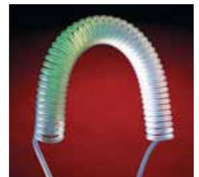
Through a proprietary manufacturing process, ZEUS "heat sets" fluoropolymer tubing into a helical coil that allow for a high degree of flexibility and retractability. This heat setting process fuses the tubing into the helical formation and allows the material to stretch and retract to its programmed position. Custom sizes, coils, and colors can all be manufactured to meet the requirements of your application.
